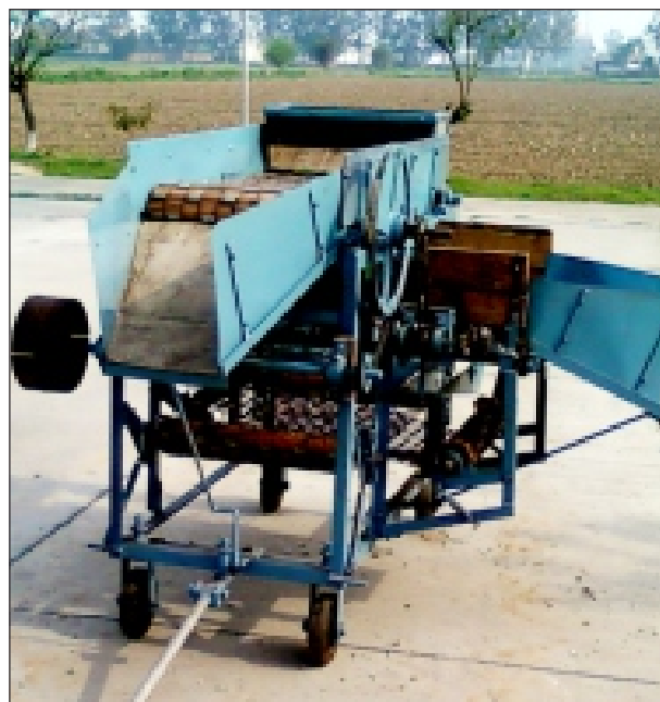
Fig. 12. Small grader for experimental plots and for small farmers
